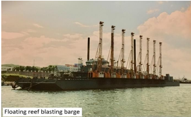
Floating reef blasting barge
